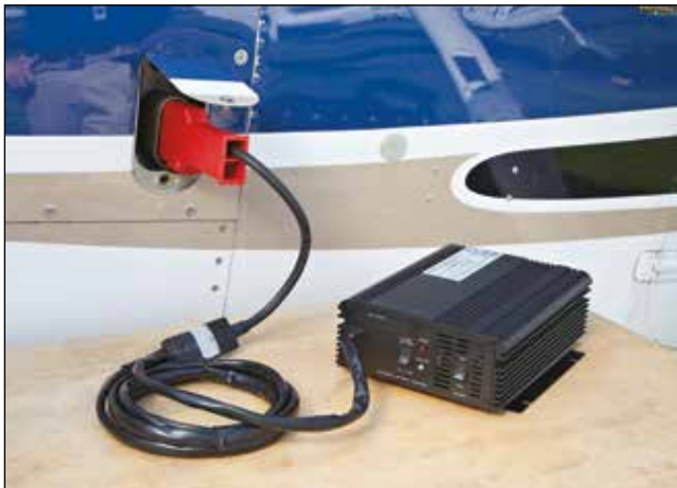
The 10.6-pound StartStick model, top, has a 9.7 Ah capacity and utilitarian display. That's the $449 28-volt Schauer power supply (sold by Sporty's) at the bottom.
